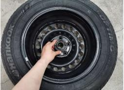
STEP 3: Place the cone on the shaft.
