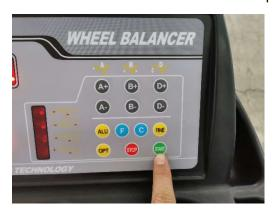
STEP 8: When the spin is finished and the wheel stops, the display will read "Add 100" (3.5 ounce). Rotate the wheel until all the outside weight indicators are fully lighted. Apply the 100 gram (3.5 ounce) calibration weight on outside edge of the rim at 12 o'clock position.
