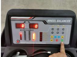
STEP 7: When the spin is finished, the display will read "0 100" (3.5 ounce). Rotate the wheel until all the outside weight indicators are fully lighted. The 100g (3.5 oz) weight should be at 6 o'clock position.
