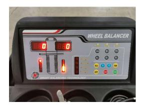
STEP 6: Apply the 100 gram (3.5 ounce) calibration weight on outside edge of the rim at random position. Press the "START" button and spin the wheel.
