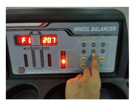
STEP 6: Press "A+" to confirm. Displays "POS 28"
