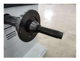
STEP 4: Next, place the wheel on the shaft. Finally, place the Quick Nut on the shaft with
