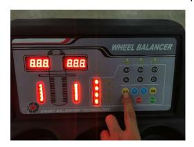
STEP 3: Manually rotate the shaft to "POS 28", press "Start" to confirm. "F1 XXX" displays.
