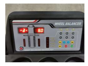
"D" (diameter of the wheel in inches. Refer to marking on tire)
