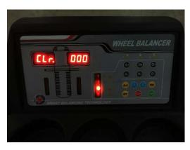
STEP 8: Press "Start" again and shaft will spin automatically and machine calculate the shaft imbalance. After the spin machine flash "End Clr" and finally display "POS xxx"
