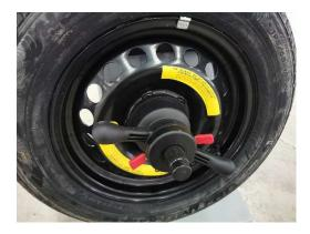
STEP 5: Verify that the balancer is in DYNAMIC mode, then manually measure and enter the parameters.
