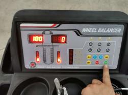
STEP 5: When the spin is finished, the display will read "0 0"
