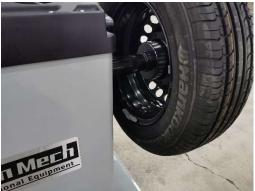
STEP 4: Remove the calibration weight from the inside edge of the wheel. Press the "START" button and spin the wheel.
