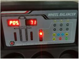
STEP 9: Press "Alu" and machine screen displays "66 67" (This is piezoelectric sensor signal, when your hand press on the shaft, the value will change dramatically. These sensors are responding to pressure force.
