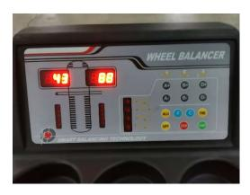
STEP 10: Press "Alu" and machine return back to working interface.
