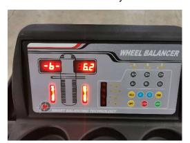
STEP 6: Enter the factory-calibration mode by pressing "F" and "C" at the same time.
