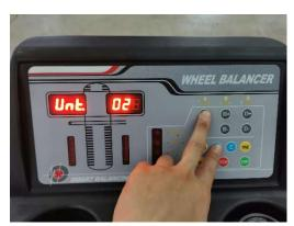
STEP 4: Set up complete and machine will automatically return back to working interface. If there is displayed value, it will be automatically switched to ounce.
